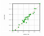
*Figure 1: Hardenss over* C<sub>stat</sub>: *Correlation coefficient 0,97.*
